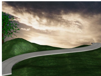
Figure 11-41 The road (Wrapper object) over a hilly area (Wrap-To object) before using the Conform tool
